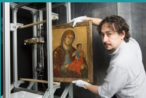
Slotting a painting into the X-ray scanner, which will analyse it at a high resolution. (Image: InsightArt s.r.o.)
